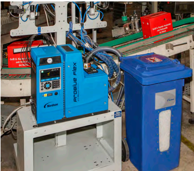
The closed hotmelt application system: the ProBlue Flex melter with MoD version fed from a 240-liter reservoir.
