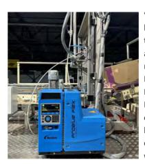
"The ProBlue Flex Melter has a modular design so that it can be individually adapted to the user's requirements," explains Erik van Gulik, OEM & Key Account Manager at Nordson. The device is characterized by a fast heat-up time and can optionally be equipped with an adhesive tracking
