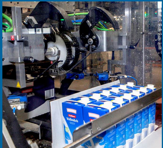
12-packs packed in wrap-around trays on their way to the high-bay warehouse
