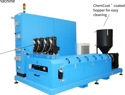
Extruders are commonly used for applications where polyamide or polyester based adhesives are processed. These adhesives need a closed system to avoid degradation degradation of the adhesive through carbonization and to provide a safe, reliable application process.
