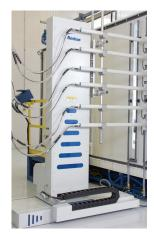
For in/out positioning of guns, features include user-programmable presets for lancing, contouring, and positioning based on part depth, shape and width. Automatic gun-mover control provides additional application flexibility and greater film-build control.
