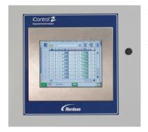
Application parameters include flow and atomizing air, electrostatics settings, and settings for gun triggering.
