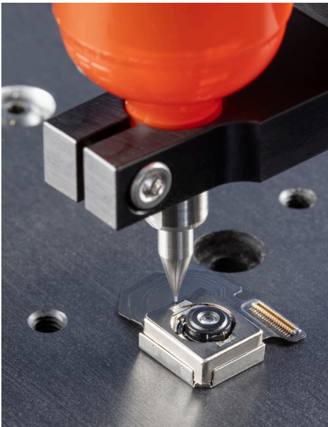
Micro-deposit dispensing onto a compact camera module.
