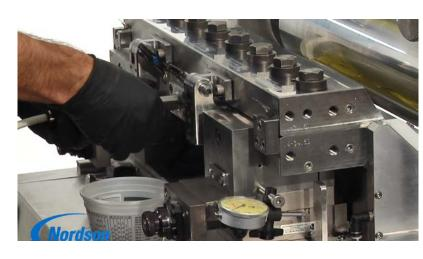
Once the feed adaptor has been removed, you can begin to loosen and remove the top bolt of each offset block. These bolts can be placed in a small bin so they remain clean and easily accessible at the time of reassembly.
