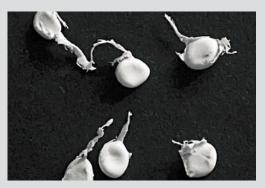
For BKG® AH and AH D pelletizers, using the die grinding tool can help remove any grooves in the die. Maintaining the blades will also help to eliminate tails on the pellets. Most pelletizer manufacturers have self-sharpening blades and this can be done while the pelletizer is in operation.
