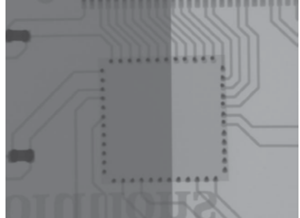
Image J: Image of flip chip with 100 µm thick zinc foil under the left half of the device.
