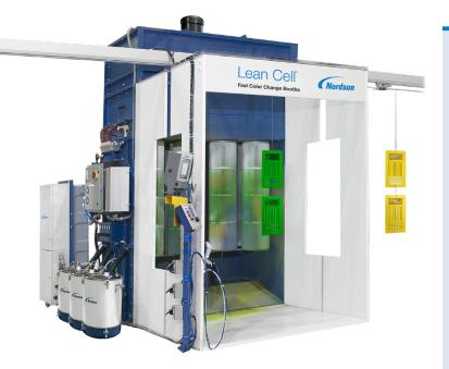
Nordson's Lean Cell conveyorized powder spray booth provides a flexible and efficient design for just-in-time manufacturing. Capable of 20-second contamination free color change with integration of Encore HD COD systems.
