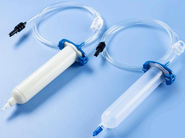
Nordson EFD's disposable Unity™ HiTemp™ syringe barrels provide a cost-effective alternative to syringes commonly used in pneumatic dispensing of hot melt adhesives. The barrels are compatible with Nordson's Unity IC Series and Unity PURJet™ 30 dispensing systems and other standard industry hot melt dispensers.
