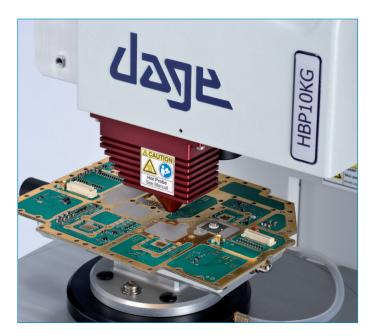
The new Nordson DAGE 4000*Plus* HBP system is a totally industry unique solution, conforming to IPC-9708 as well as JEITA ET-7407A. It is fully integrated into a single load cartridge on a standard 4000*Plus* system. Heating, cooling stages and pin clamping mechanism are integrated into the single load cartridge. The Paragon<sup>™</sup> software provides a user friendly interface via temperature time profiles to setup a test.
