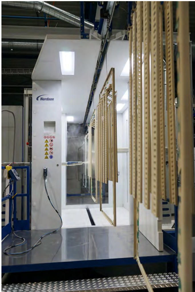
Soft spray from the Encore HD spray guns ensures full coverage in corners and recesses.
