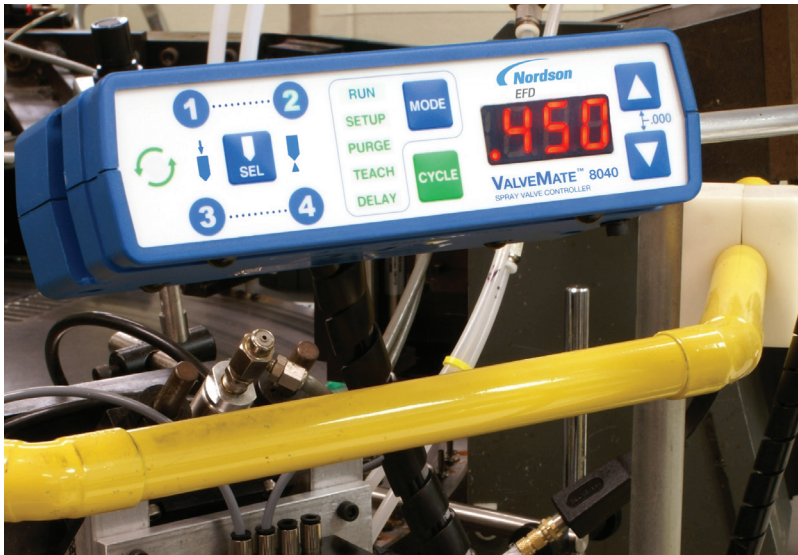
The ValveMate 8040 controller is a fast, convenient way to adjust spray valve open time in increments as small as 0.001 seconds.
