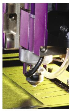
Figure 2. Jetting technology enables surface mount adhesive to be applied after solder paste without disturbing the paste.
