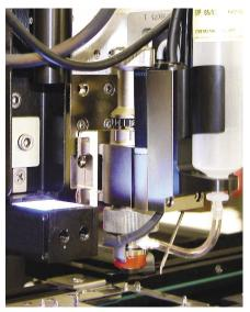
**Figure 1.** A pneumatic piston impels fluid through a narrow orifice at the end of the nozzle.
