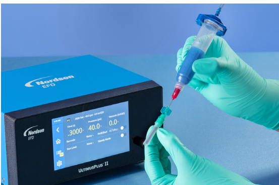
Class VI components dispensing onto a catheter.
