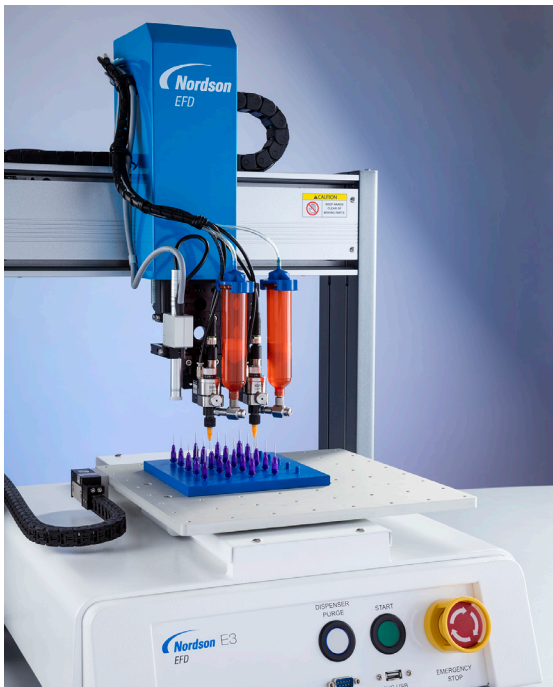
An EV robot dispensing UV material onto medical components.
