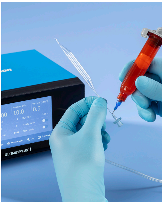
UltimusPlus simplifies set up for catheter bonding applications while providing better process control for higher product quality.
