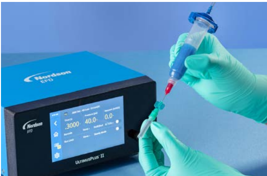
Class VI components dispensing onto a catheter.
