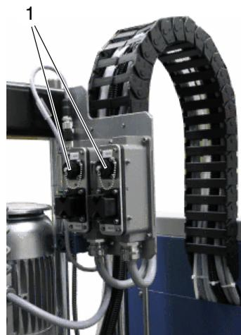
Connect the assembly handgun switches to receptacles Hose/Applicator 1 and Hose/Applicator 2.
