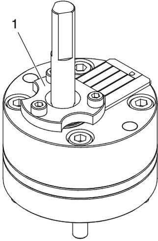
*Variseals* are fixed in place on the pump with a flange (1). If material escapes along the shaft, the pump shaft seal must be replaced.
