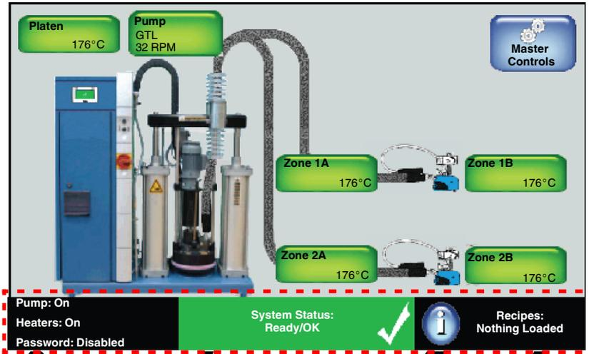
View (only) the state of the Master Heater and Pump controls, as well as whether or not password protection is enabled.
