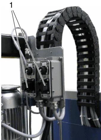
Up to two hoses can be attached to the platen. Guide the hoses through the hose holders to the platen and initially connect them electrically to interfaces Hose/Applicator 1 and Hose/Applicator 2 .
