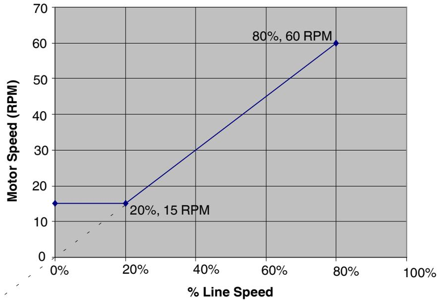
Figure 6-3 Gear-to-Line, single-point on a curve
