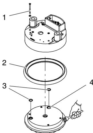
1. Heat the platen until the material softens (approx. 70 °C / 158 °F, depending on the material).
