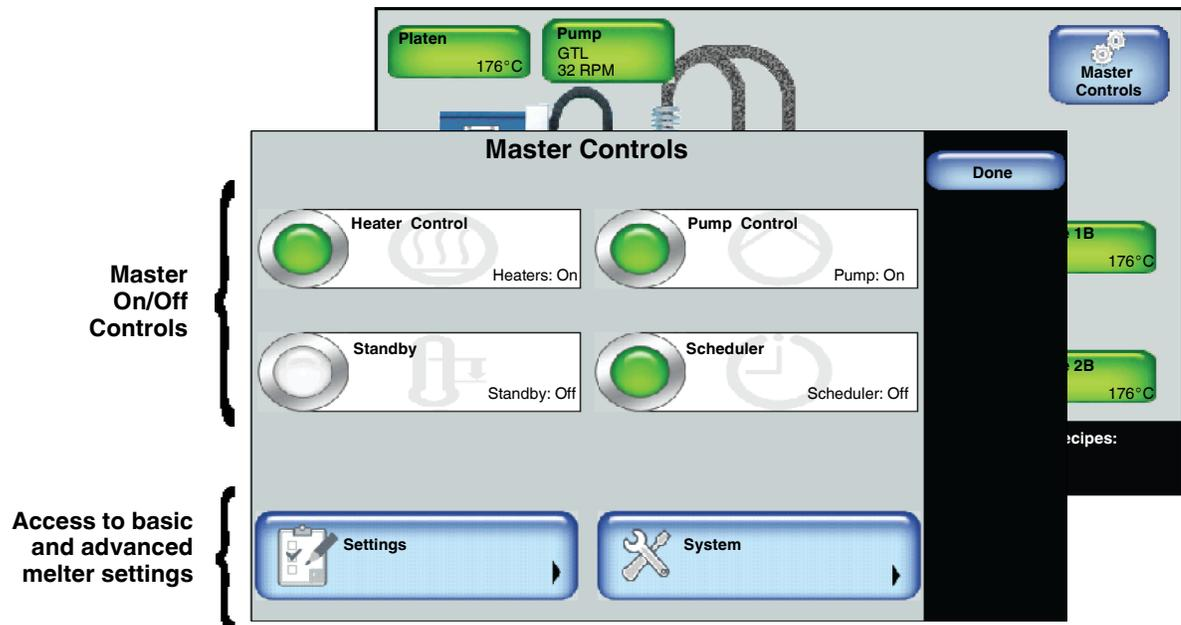
Figure 5-2 The Master Controls Display
