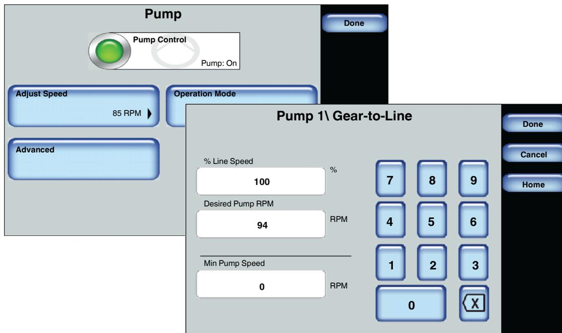
Figure 6-4 Configuring and adjusting Gear-to-Line mode
