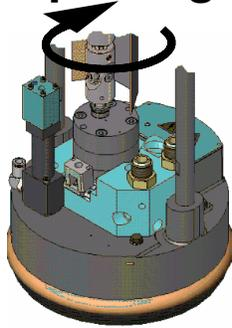
**NOTE:** Perform work only when the material is soft (approx. 70 °C/158 °F, depending on material); otherwise the Cardan joint can not be turned.
