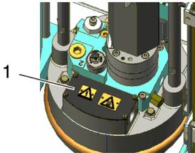
1. Disconnect the bulk melter from the line voltage.
