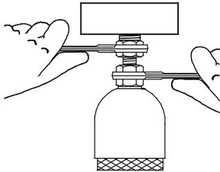
To prevent the hose connection from turning, use a second open-end wrench when connecting and disconnecting the hose.
