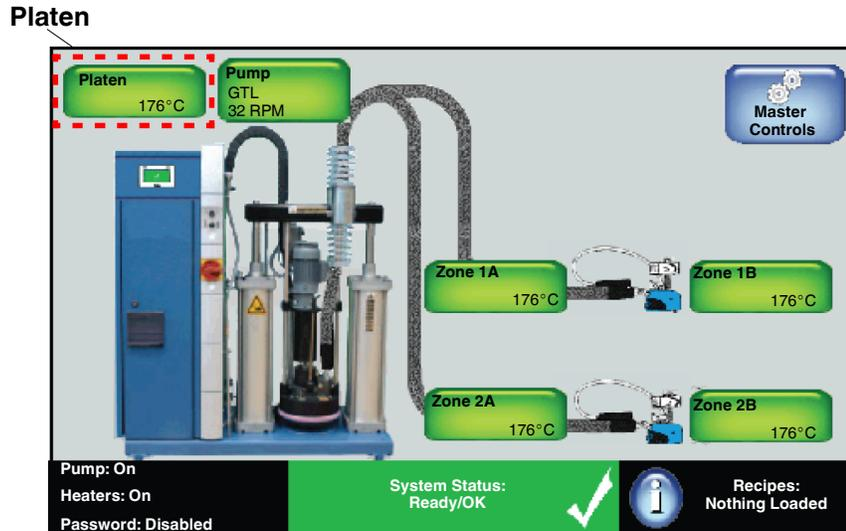
From the **Home** screen, you can view the state and status of the platen. Touch the **Platen** button to do the following tasks:
