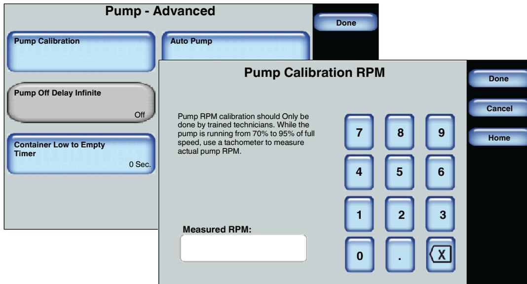
1. Wire a tachometer to the pump.
