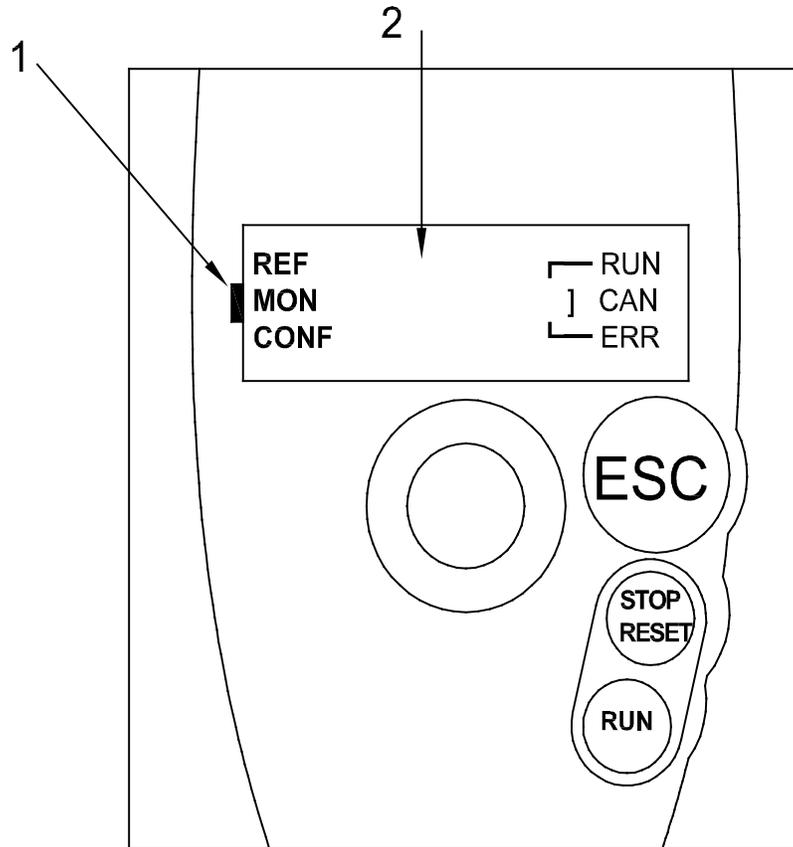
Figure 9-1 Motor drive power LED and display
