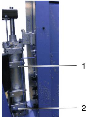
A switch rod activates the two switches (1 and 2) one after the other, triggering the following switching functions:
