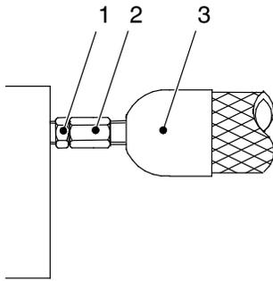
If cold material can be found in the hose connection (1), the components (2, 3) must be heated until the material softens (approx. 70 °C / 158 °F, depending on material).
