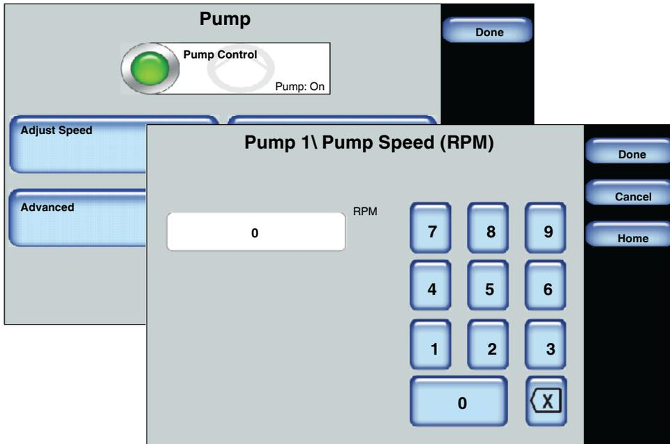
Figure 6-5 Configuring and adjusting Manual mode
