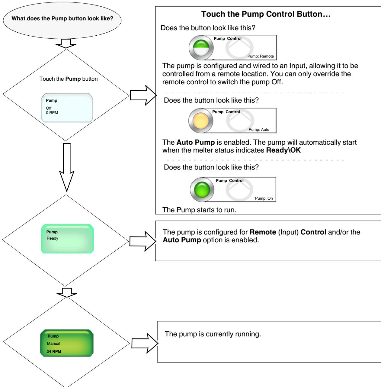
Figure 6-2 Getting the Pump to Run
