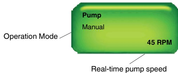
Figure 5-4 Pump button details
