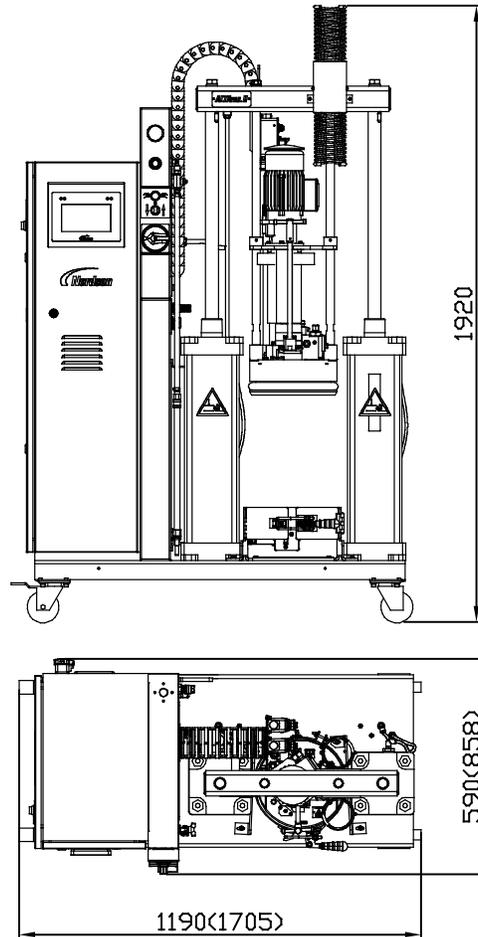
Figure 12-1 Dimensions in brackets: Space required for installation
