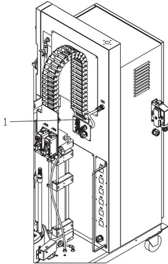
Connect dry, clean and non-lubricated compressed air to the compressed air connection (1). Dirt particles in the air may not exceed 30  $\mu\text{m}$  in size.
