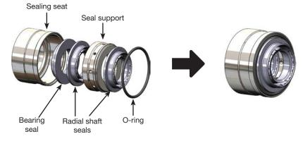
2. Install the seal bearing assembly on the rotor assembly.
