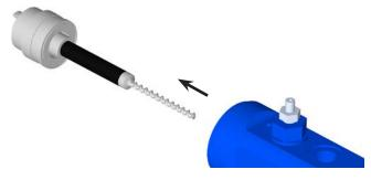
4. Carefully isolate the seal bearing assembly from the rotor assembly.
