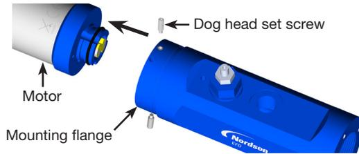
2. Unscrew and remove the mounting flange.
