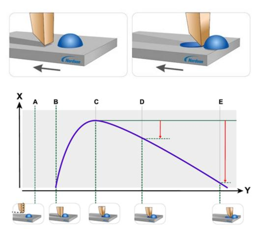
The shear tool position during testing is critical for accurate and repeatable test results. Nordson DAGE cartridges find the device surface using an sensitive touchdown feature. High precision positioning provides shear height accuracies of +/- 0.25 microns. Touchdown is achieved using a patented load cartridge clamping system which ensures every bond is sheared at the same height relative to the surface that it is bonded on.
