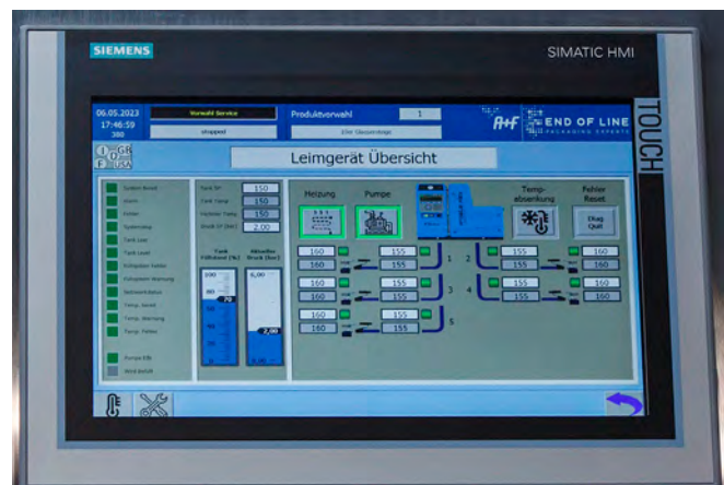
The controller is integrated into the HMI of the parent machine.
