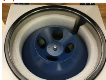
Incorrect: No rotor sleeves or adapters used; retained foam insert
