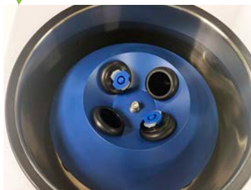
Correct: Axially symmetrical placement of two barrels
