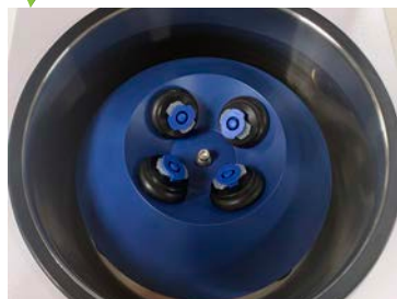
Correct: Four barrels loaded using the correct adapter size
