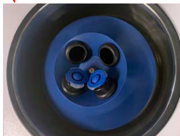
Incorrect: Wrong size adapters used, thus creating interference
