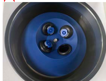
Incorrect: Three barrels loaded
