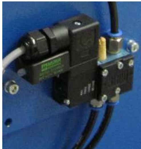
Fig. 2-12 Solenoid valve (left) - pressure relief valve with container
