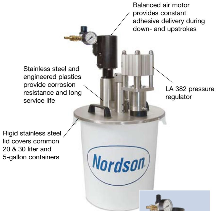
Nordson LA 310 dual-acting piston pumps offer flexibility and consistent flow rates of liquid adhesives in folding carton, envelope, and bag and sack manufacturing. Whether lid-mount or wall-mount versions, or on Nordson's adhesive system console, the system offers flexibility for installations in OEM machines or to retrofit existing production lines.
