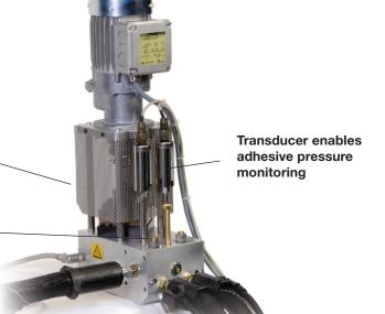
Stations potentially eliminate need for additional melter and increase adhesive delivery points
