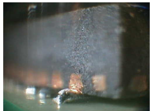
Images 7 & 8: Optical images of a QFN showing that solder joints have formed on the base of the device. However, if the side terminations do not wet then the visual appearance of the joints may vary making it very difficult for AOI inspection. The land pattern should still extend outside of the component footprint and the length of the pad designed under the part should extend to the end of the metalisation. Although good wetting of the side terminations is not required to make a good QFN edge joint, if they are present then it is often a great help to inspecting their quality in the real world of manufacturing.
