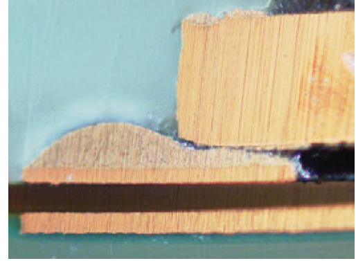
Image 6: Micro-section of a QFN on a flexible circuit. The QFN has 'floated' due to excessive paste deposited on the central pad and/or excessive voiding in the centre pad. This has caused an open joint. This failure may have been exacerbated by solderability or burring issues in the component plating.
