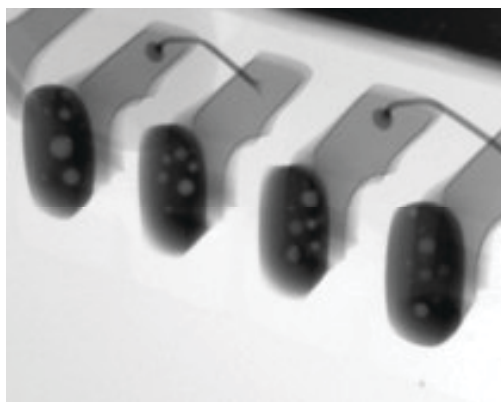
Image 16: Acceptable Condition of QFN edge joints showing an increased level of voiding within the joints but well within any action level.
