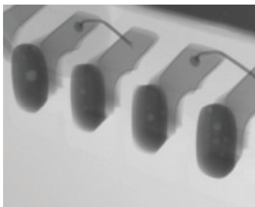
Image 15: Target Condition of QFN edge joints where showing a moderate level of voiding within joints is acceptable. All joints have reflowed.
