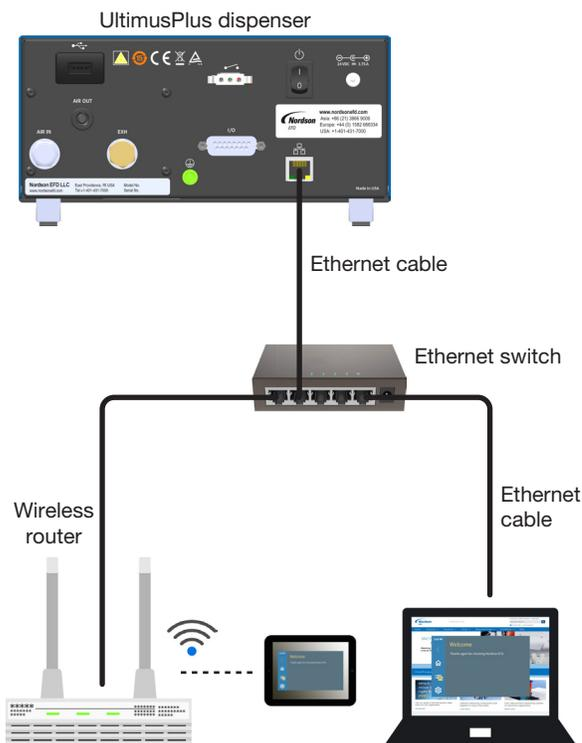
*NX web interface open on a tablet and a PC connected to an UltimusPlus dispenser*
