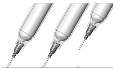
**Remember** — always bring the tip in contact with the work surface at the illustrated angle. After the tip is in position, press the foot pedal. Release the pedal and remove the tip by lifting straight up.
