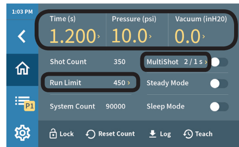
Editable settings on the Home screen: Time, Pressure, Vacuum, Run Limit, and MultiShot
