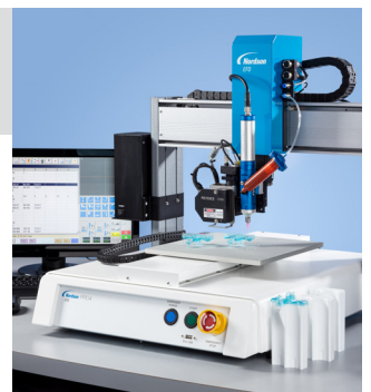
The PROPlus dispensing automation solution provides repeatable fluid application in simple to complex patterns.
