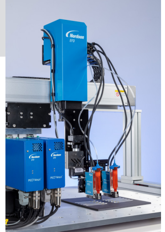
Small form factor makes it easy to mount multiple controllers on a DIN rail.
