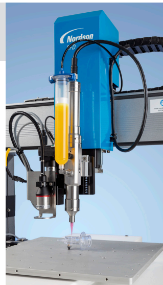
Nordson EFD's stainless steel progressive cavity pump offers a corrosion resistant dispensing solution for manufacturers looking to maximize the longevity of their capital equipment investments.
