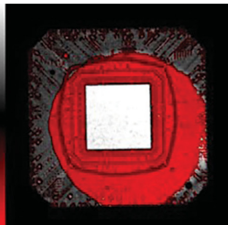
Figure 2. Acoustic identifying defects.
