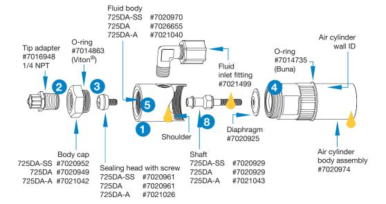
NOTE: Before reassembling the valve, clean all parts, and replace the O-rings, sealing head, and diaphragm.
