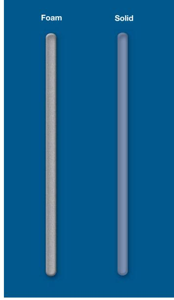
Foam produces the same volume at up to 50% less weight than solid material.
