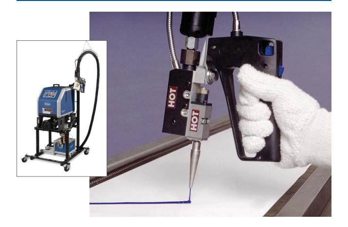
Hot melt materials are commonly used in automotive assembly for bonding of sound deadening material (shoddy pad), carpet, foam blocks and fabrics to various types of plastics, compressed wood and fiberglass. The material, including EVA, polyamide, APAO and pressure sensitive-based products, can be applied as a bead or in a swirl spray to meet specific application requirements.
