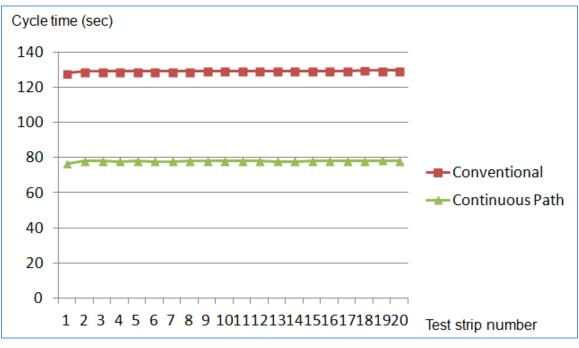
Figure 5: Cycle Time Difference in 20 Strips Between Conventional & Continuous Path Motion Control
