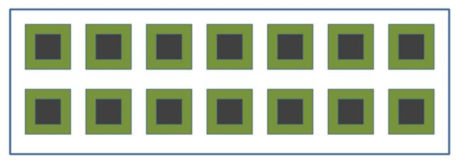
Figure 1: 2 x 7 Boat Die Layout for Traditional Flip Chip
