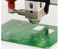
Non-contact micro-dispensing of beads and fills onto hard-to-access or delicate surfaces is easy and repeatable.
