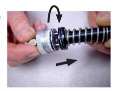
4. Install the air cylinder cap, piston and spring by pushing to compress the spring while turning to engage the threads.
