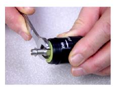
9. Remove the shaft and diaphragm.
