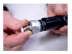
5. Using the two 8" adjustable wrenches, tighten the air cylinder cap. If a torque wrench is available, torque to 10.8 Nm (8 ft lbs).
