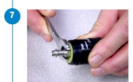
8. Insert the 1/8" hex wrench through the air inlet fitting and tighten the shaft locking screw. If a torque wrench is available, torque to 2.82 Nm (25 in lbs).
