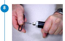
9. Install the fluid body and tighten using the 1/8 NPT rod and 8" adjustable wrench. If a torque wrench is available, torque to 6.78 Nm (5 ft lbs).
