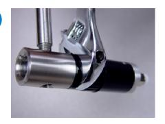
6. Remove the fluid body from the air cylinder.
