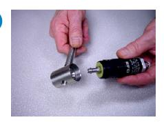
7. Insert the 1/8" hex wrench through the air inlet fitting, loosen the shaft locking screw, and turn it out two full turns.
