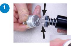
2. Using the lubricant supplied in the repair kit, apply a film of lubricant to the points indicated.
