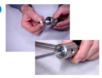
11. Install and tighten the fluid body cap using the 1/8 NPT rod and 8" adjustable wrench. Remove the 1/8 NPT rod.
