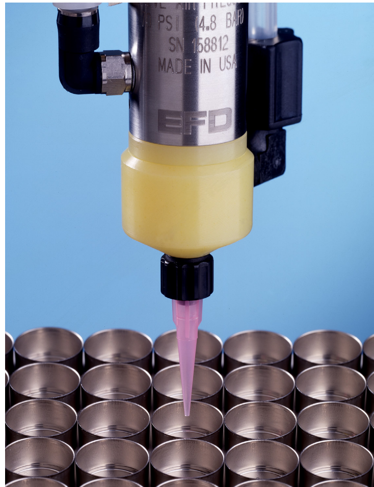
Nordson EFD's precision filling systems provide an automated solution for filling and topping off applications.
