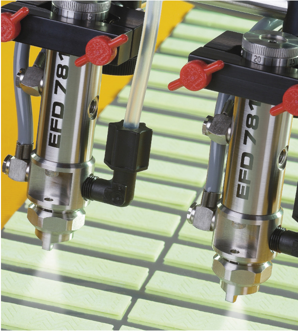
781 spray valve coating sugar on gum.
