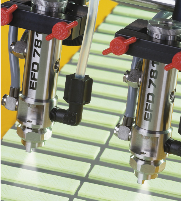
781 spray valve coating sugar on gum.
