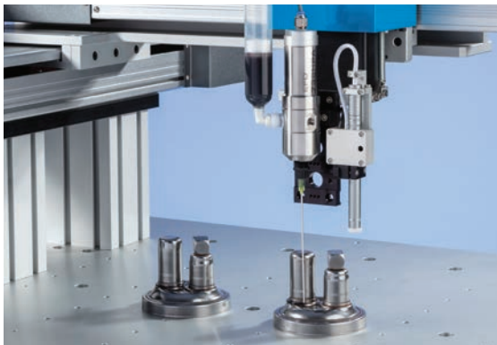
The 736 valve dispensing grease onto automotive fuel pump bonnet.
