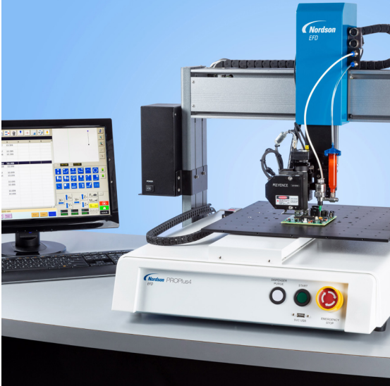
PROPlus Series automated dispensing robots feature best-in-class positional repeatability of +/- 0.003 mm (3 µm).
