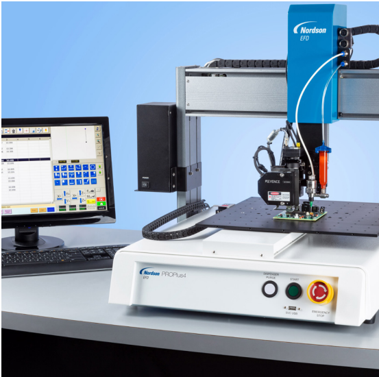
PROPlus Series automated dispensing robots feature best-in-class positional repeatability of \pm 0.003 mm ( 3\text{ }\mu\text{m} ).
