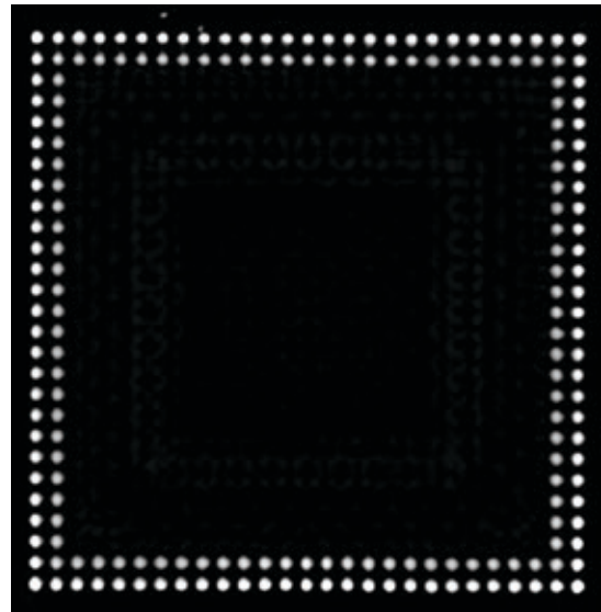
Figure 9. Fast, low magnification PCT scan of POP device in figure 8. The virtual cross section through the plane of layer 1 looks consistent and good.
