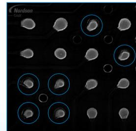
Head in pillow and open joints (see blue circles) effortlessly identified using X-Plane<sup>®</sup>.
