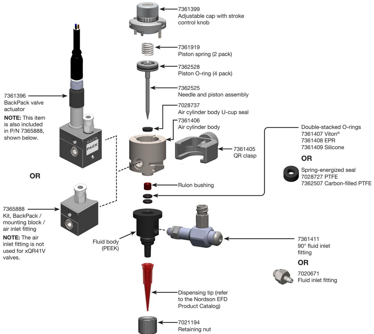
xQR41V valve replacement parts (valve with double-stacked O-rings shown)
