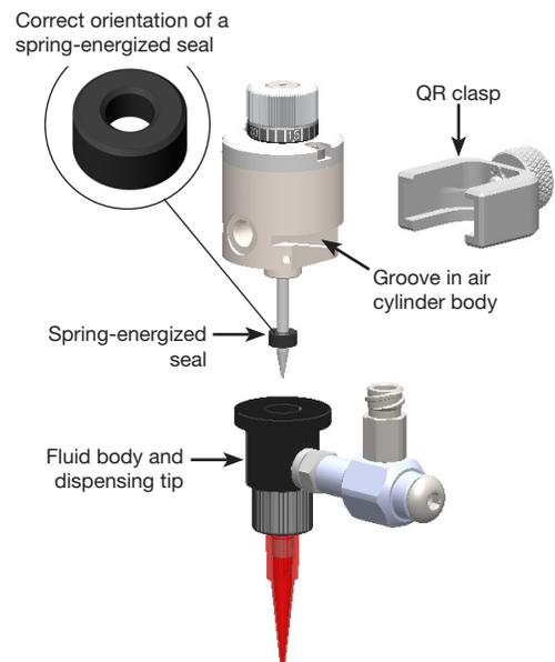
*Fluid body change of a valve with a spring-energized seal*
